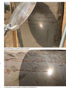
CERAMIC PLASTER AFTER SINTERING
